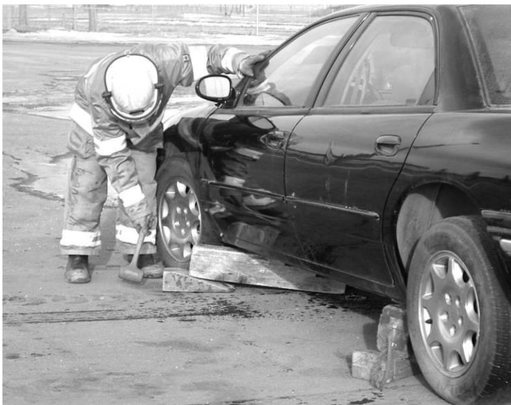
***A Wedge under Each Step Block Will Tighten the Block against the Underside of the Vehicle***
