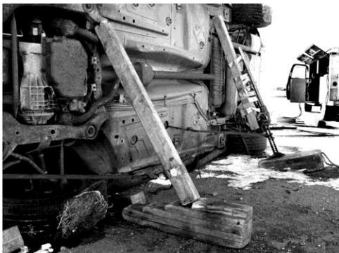
***A Jack-All, 4x4 Posts, Straps and Wedges Have Been Used To Stabilize This Vehicle from the Undercarriage***
